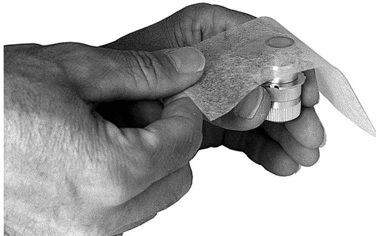
**Figure 8-1: Cleaning a Mirror Surface**
