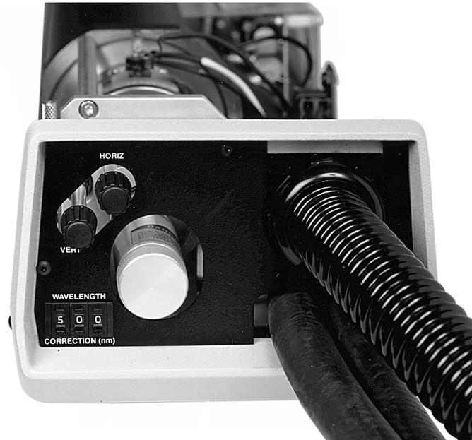
Figure 4-2: Laser Head Control Panel
